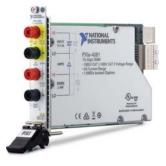
National Instruments has announced the NI PXIe-4081 7 -digit high-performance DMM and 1.8 MS/s isolated digitiser. The NI PXIe-4081 is the first PXI Express DMM available. It offers engineers the resolution flexibility, and isolation needed to tackle challenging applications that require smarter test systems in industries ranging from consumer electronics to aerospace and defence.
