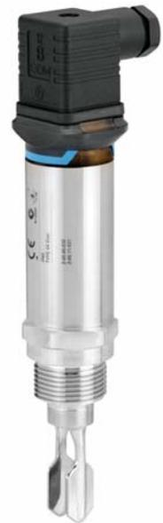
The Liquiphant FTL31 and FTL33 liquid level switches, from **Endress+Hauser**, are based on vibrating tuning fork technology. The sensors are excellent replacements for float switches or conductive, capacitance and optical sensors. The FTL31 is designed for the chemical, oil and gas and other Industries, while the FTL33 is
